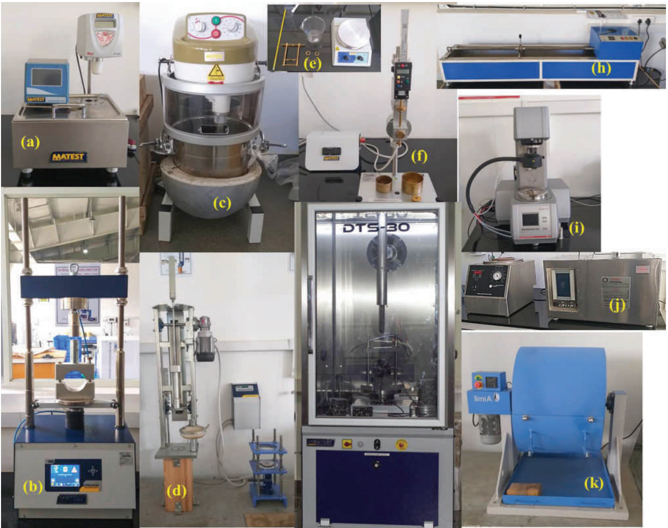
Equipment in Advanced Pavement Systems Laboratory at IIT Tirupati:
