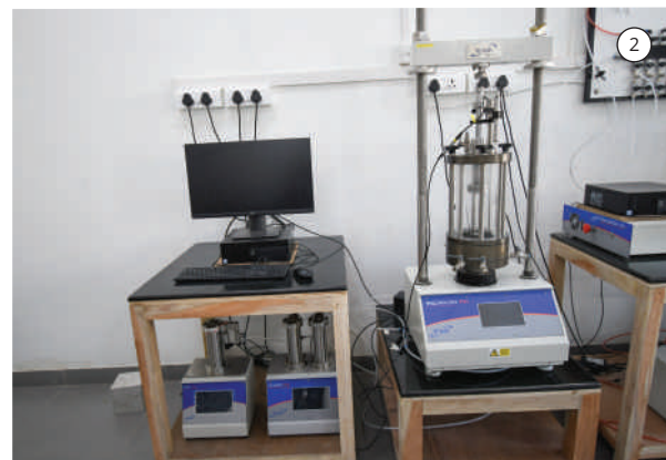
100 kN load frame for large size triaxial testing
