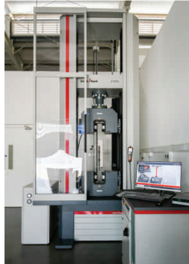
High capacity Electro-mechanical UTM in Structural Engg lab
