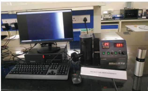
Millikan's Oil Drop apparatus to determine the charge of an electron
