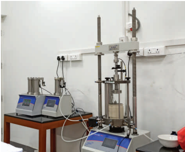
Automated stress-path static triaxial apparatus with permeability measurement
