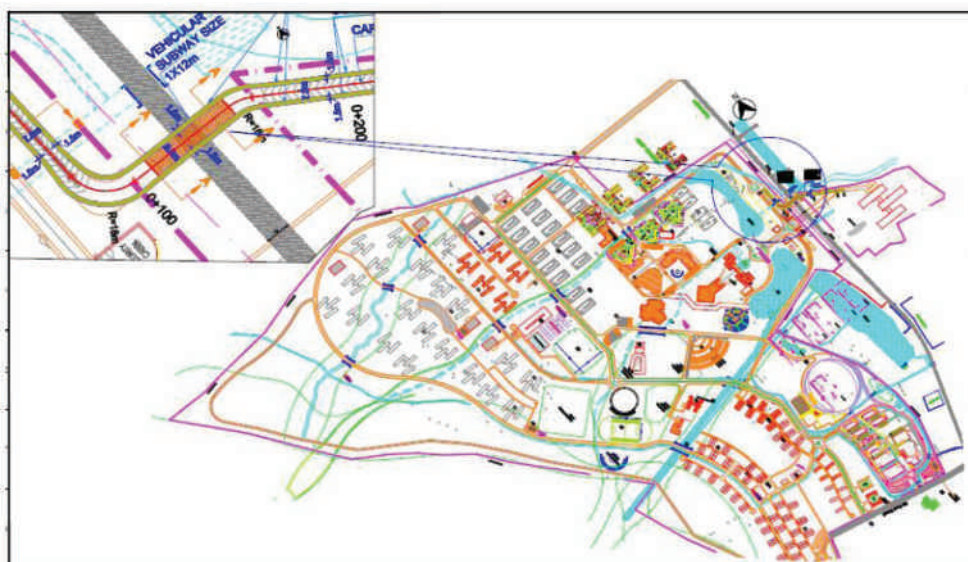
Typical plan showing the underpass connecting the two parcels of the campus on either side of NH-565
